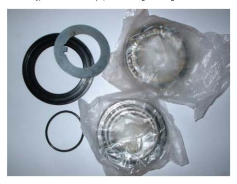
Back to business...Remove the hub oil seal by levering it out using a pry-bar, or a big screwdriver. Remove the inner bearing and clean all the components carefully. Inspect the bearings and race very carefully, any sign of scoring, or wear on the tracks; or any signs of grittiness when the bearings are run on the races, then the bearings must be replaced. If one is okay, and the other isn't, replace them both. Replacing just one is false economy.
