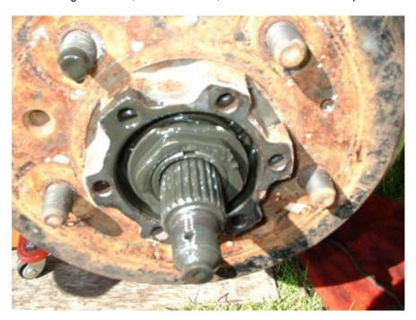
Now undo the three screws holding the brake drum in place, and pull off the drum. Don't forget to back off the brake adjusters first!
