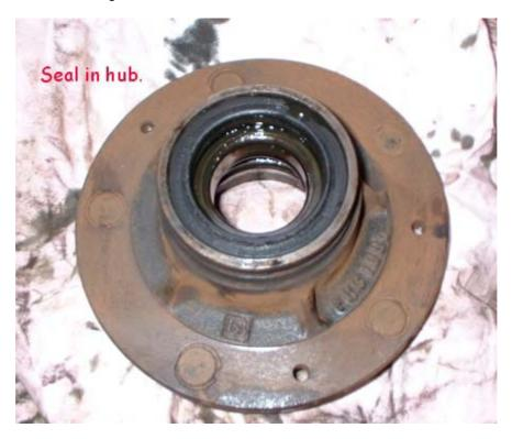
You might use a big socket or similar for this, but it is important that the seal goes in evenly, and the lips are not damaged. The later type of seal, with two lips, as fitted to 1980 onwards axles should fit so that the outer of the lips is about 1mm below the hub casing. It has a lip on the outer edge of the seal too, and this should end up flush with the hub casing.
