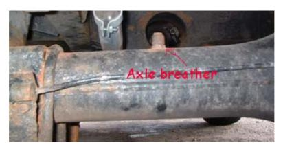
Remove the brass bell-shaped fitting on the top of the axle, and give it a shake. There is a ball bearing in there, which will rattle if the breather is not completely blocked with dirt, if it does rattle, try blowing through the breather, as sometimes the outer part can be blocked with dirt, even if the ball bearing rattles inside. It is possible to clean them out with a bit of wire and some petrol, or WD40, though. It just needs a bit of patience!
