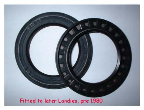
Now a look at the later type of seal, as fitted to axles made after 1980, again, the top seal is showing the inside (i.e. facing the inner bearing)
